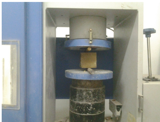
Figure 5. Indirect tension test for polyester mortar cubes.
