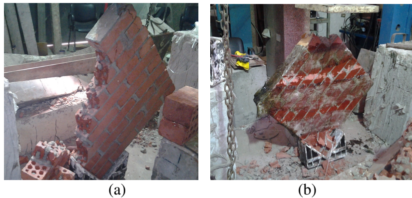
Figure 6 Failure modes for a) control wallets, b) FRP-strengthened masonry wallets
